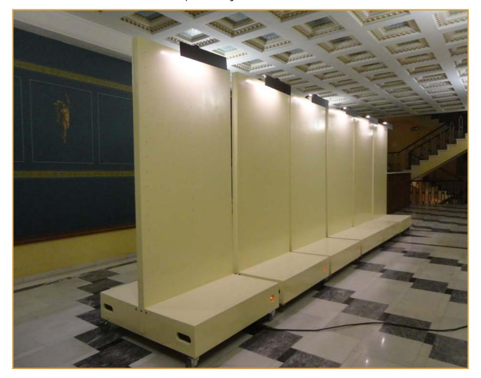
The stands were made by lacquered MDF & sheet metal and were designed to dismantle for easier transportation. The Frames could be hanged by special plugs and posters with magnets. All the stands could be linked together to avoid multiple power wires. An electric diagram was glued underneath each stand to ensure that connections would be understood by any kind of technician.
